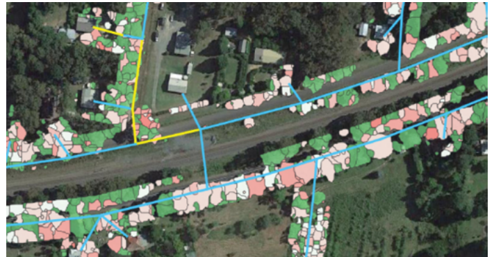
Top: Vegetation canopies separated out in LiDAR data. Bottom: Tree fall-in defects per span using predictive modelling
